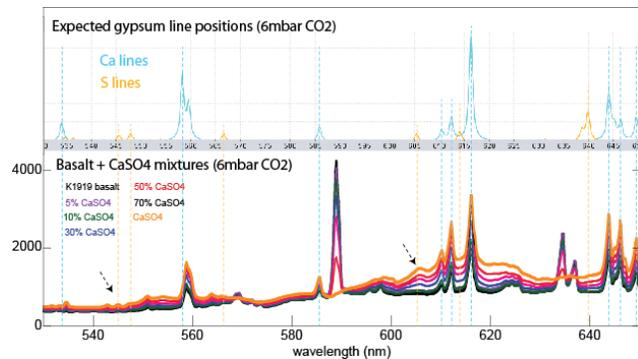
Figure 2. (top) location of Ca and S lines expected under Mars pressure [16] (bottom) mixtures of basalt with gypsum. Ca line intensity increases with increasing proportion of salt; however, only 2 of 5 wavelength regions (arrows) exhibit subtle emission peaks that may be related to the presence of sulfur.
