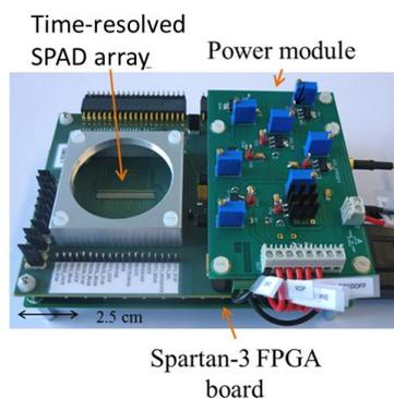
**Figure 1.** 1024 x 8 SPAD array integrated with the prototype FPGA board
