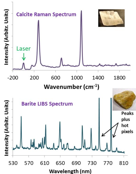
**Figure 4.** Time-resolved Raman and LIBS spectra using the 1024 x 8 SPAD array.
