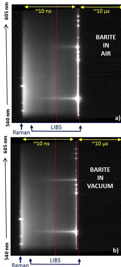
**Figure 2.** Streak camera images showing Raman and LIBS spectra of Barite in air and in high vacuum ( $10^{-5}$  mbar). The y-axis represents wavelength and the x-axis represents time. The Raman peaks coincide with the timing of the laser pulse, with LIBS occurring over a longer time scale.
