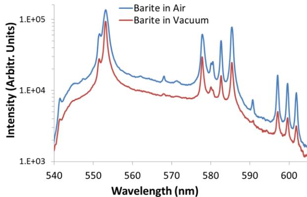
**Figure 3.** LIBS spectra of barite in air and under high vacuum ( $10^{-5}$  mbar). These spectra represent the sum of spectra within the time region between the red lines in figure 2.
